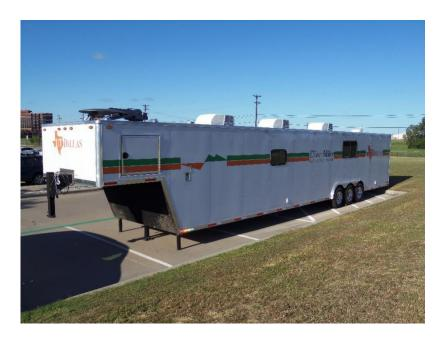
The base flooring of the unit will be aluminum (no wood) covered with a black or gray coin patter rubber flooring. The unit will be insulated with insulation in all walls and ceiling will be covered with a .40 white aluminum. Gray wall coating will be added where specified and tie down points will be added throughout the unit to secure items during transport. LED lighting will be used throughout the unit interior.
